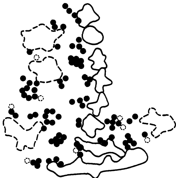
Figure 2. The same section of CPA as Figure 1 showing all non-hydrogen atoms between the helices and the \beta sheet. The heavy dotted lines enclose helical backbone atoms. The heavy solid lines enclose \beta backbone atoms. The section is effectively perpendicular to the helices and to most of the \beta sheet. Filled circles again represent side-chain carbons. Dotted circles are other non-hydrogen atoms.
